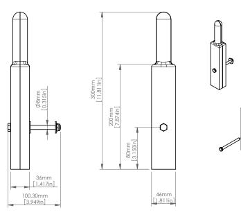
The Brake Lever is to be made from two 18mm [3/4in] thick pieces of timber nailed and glued together. The top of the Lever is to be rounded and shaped as smoothly as possibly. Use a wood chisel, file/rasp and sandpaper to shape.
