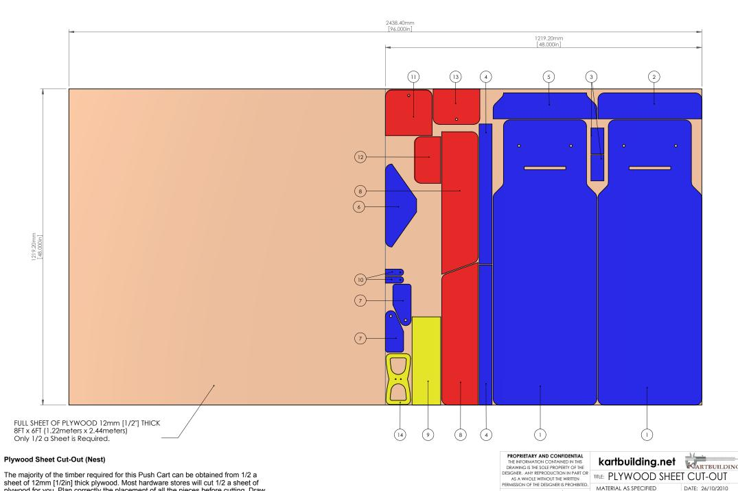
plywood for you. Plan correctly the placement of all the pieces before cutting. Draw out the pieces on the sheet of plywood before cutting with a panel saw (hand) or jigsaw (electric) or skill-saw (electric).
