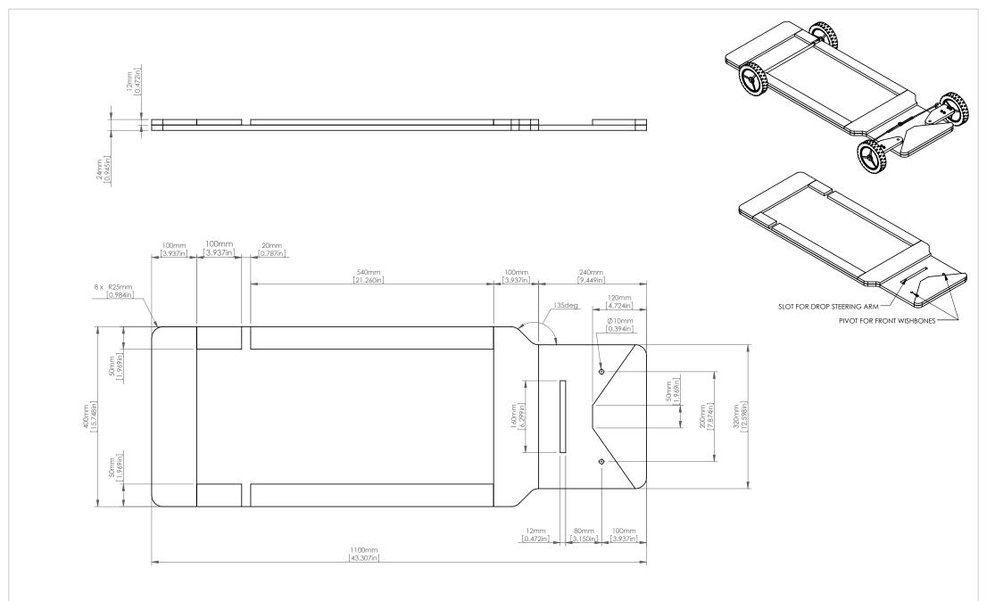
Nails and Wood Glue is used to secure all the pieces of Plywood together. If the nails protrude/stick through, bend the nails back over flat (clinch). This makes for a strong connection. You can use wood screws and glue either. Nails are generally cheaper and quicker to use.
